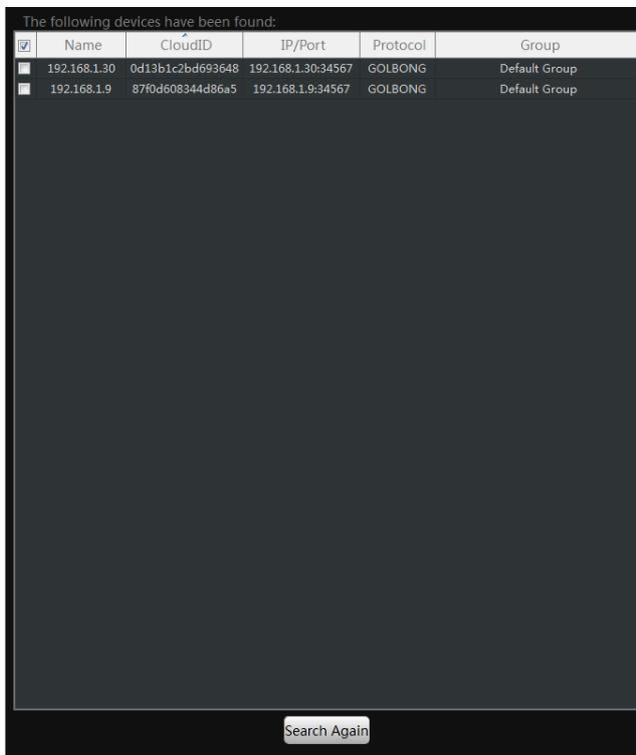
4. Mark the checkbox in front of the IP address, click “Add ” button. The IP camera will move to right.
