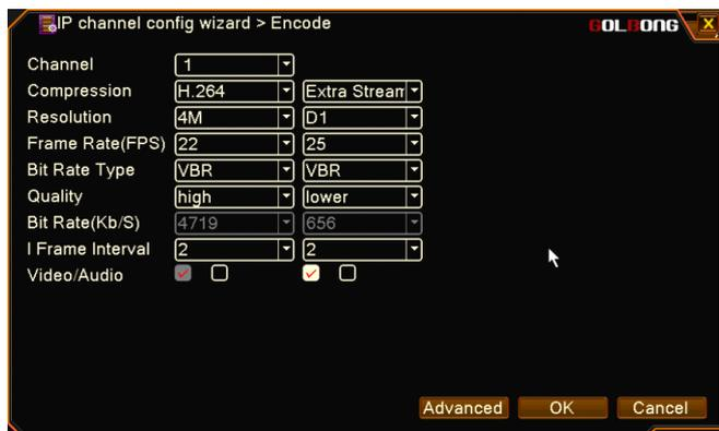
NOTE: Resolution - Main stream-preview HD/SD , and it affects the viewing quality of the video. Sub stream is more suitable for remote viewing, it can save bandwidth.
