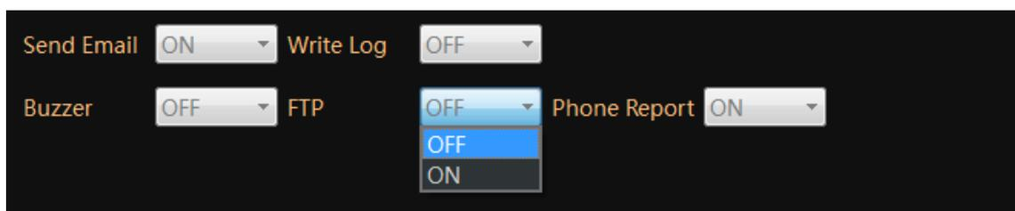
NOTE: The camera will upload the video or snapshot to the FTP server when it catch a motion detection.
