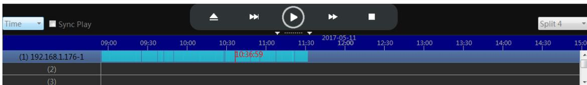
7. Move the mouse to the time frame, time will display in white. Click the mouse, the software will start playback the footage from this moment.
