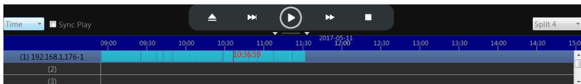
8. Move the mouse to the time frame, time will display in white. Click the mouse, the software will start playback the footage from this moment.
