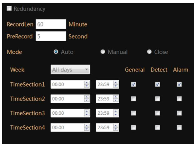
NOTE: Check "General" will keep camera recording continuously. Unchecked the "General", the camera will only record the footage when the motion or alarm input is detected. It can save the hard driver space.
