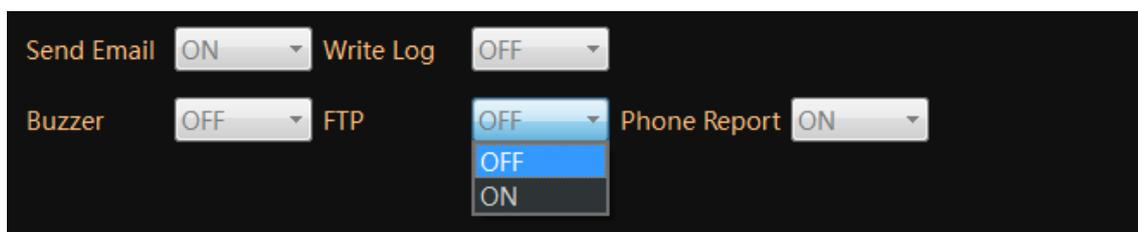
NOTE: The alarm input FTP upload requires external alarm devices such as door contact is connected to the camera properly.
