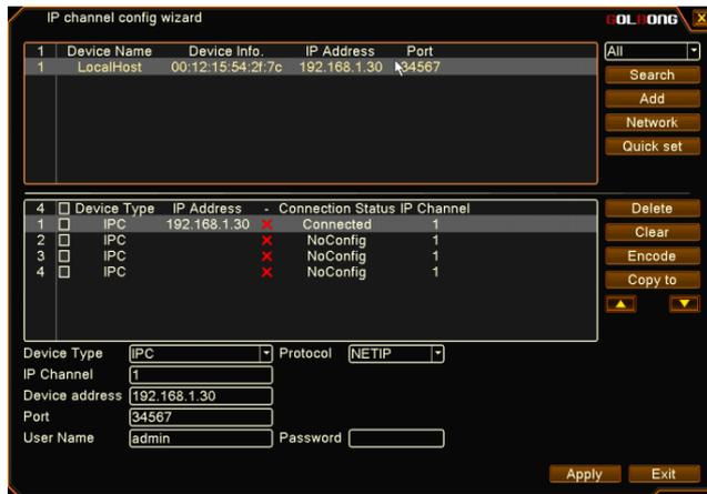
3. Press “Auto assigned”. The recorder will assign static IP address to your IP camera automatically.
