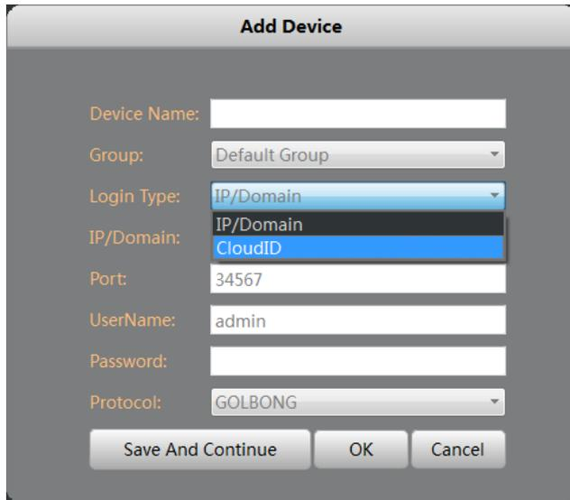
Optional 3: How to Configure the network setting of the camera manually.
