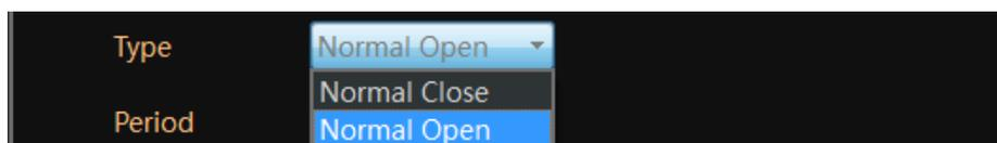
NOTE: Normal Open means the alarm device stays OPEN, it generates digital signal to the camera when the status change to closed.
