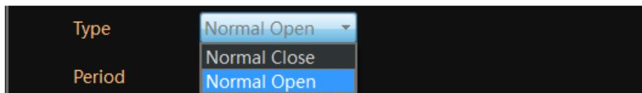
NOTE: Normal Open means the alarm device stays OPEN, it generates digital signal to the camera when the status change to closed.
